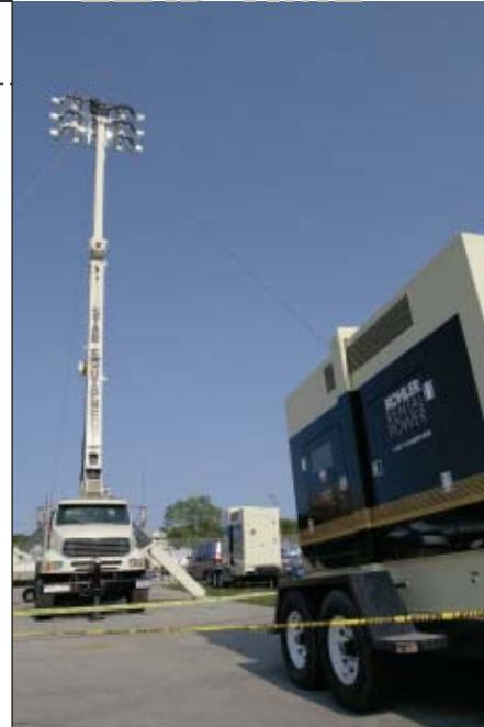
**One week prior** to the first lap, Kohler Event Services was preparing for the first Champ Car night race, supplying 14 generators ranging in size from 50 kW to 180 kW, and one 180 kW KOHLER Dual Pack.. One generator serves as the primary source, the second as a built-in back-up – ideal for applications that demand constant, reliable power.
